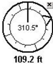
The vertical line at the top of the dial represents your direction of travel. The moving arrow represents the direction to the target. The distance to the target appears below the dial.
